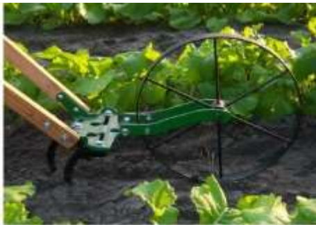
Hoss Standard Single Wheel Hoe w/3 cultivator teeth
