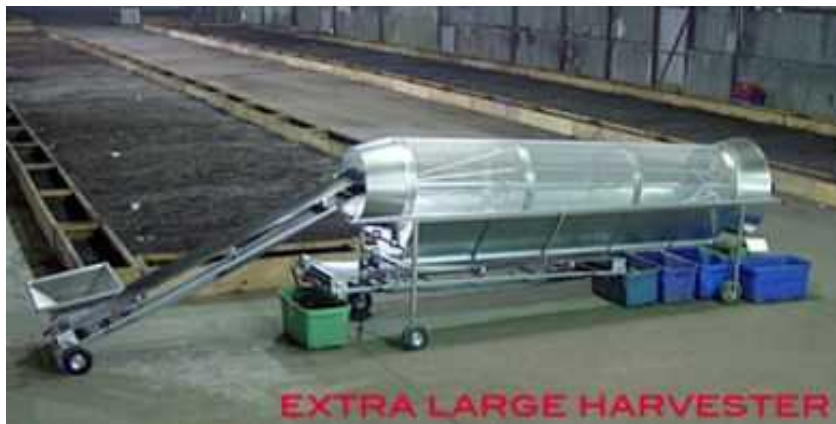
Figure 5: Commercial mechanical worm harvester. The vermicompost is added to the left end, travels down the belt, and falls through the mesh into buckets below. Worms remain on the belt and are deposited into the green bucket at the right end. Photo
