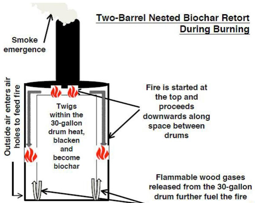
FIGURE 2. Two-barrel nested biochar retort
