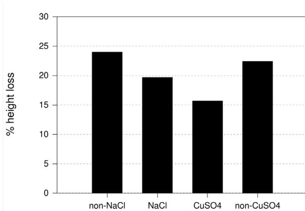
FIGURE 2. Salt-treated cobs lost less height than the untreated cobs.
