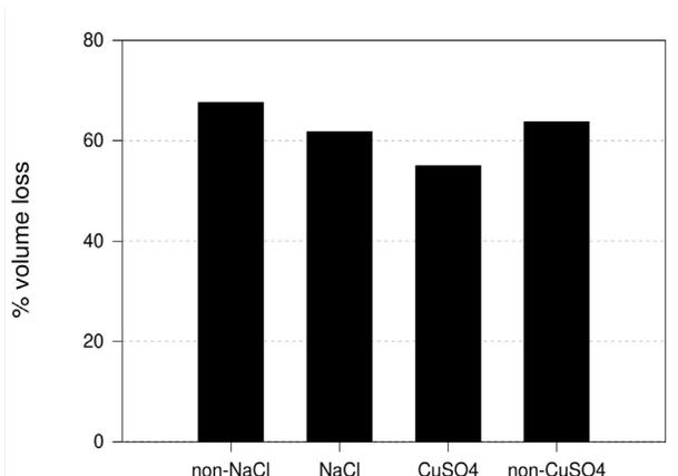
FIGURE 4. Overall, the salt-treated cobs lost less of their volume than the untreated cobs.
